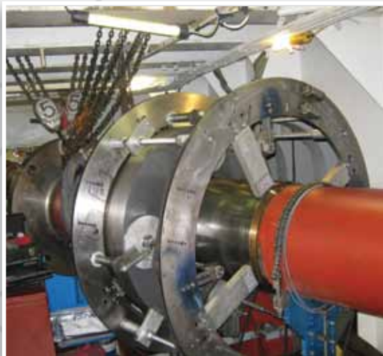
Refurbish Thrust Face on Propeller Shaft
