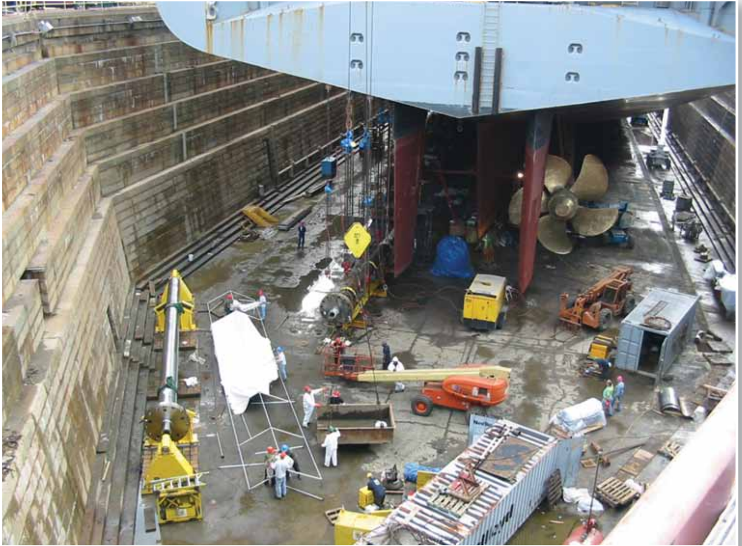
Machine Propulsion Shafts Using Portable Lathe
