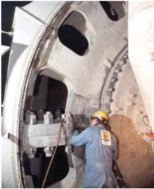
Ball Mill Metalstitch® Repair
