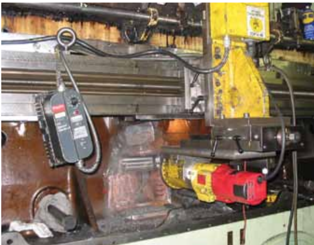
Machining Diesel Engine Insert After Metalstitch® Repair
