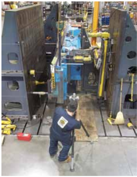
Verify Alignment During Repair
