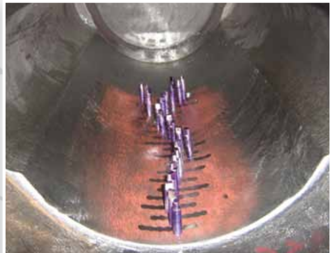
Extrusion Press Bore Metalstitch® Repair
