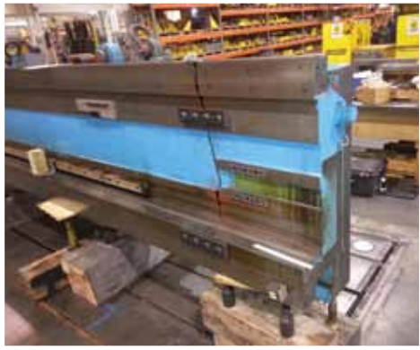
Cracked 25 Foot Gantry Mill Rail
