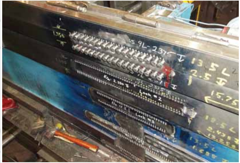
Installing Stitchescrews®, Stitchlocks®, and Masterblocks
