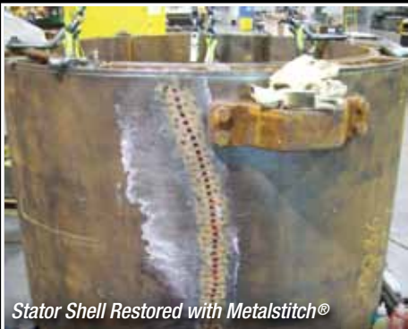
Metalstitch® Repair of Steam Turbine Shell
