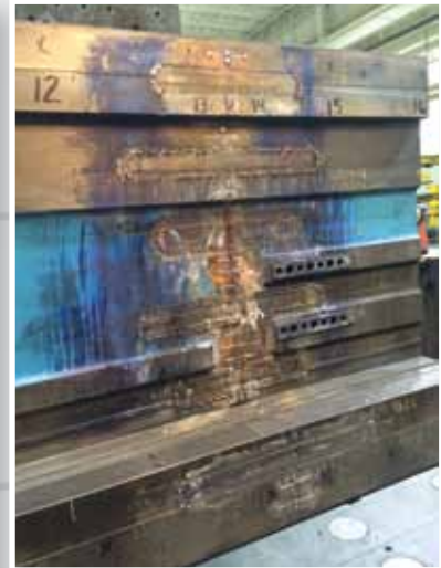
Metalstitch® Repair Ready for Machining
