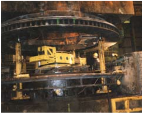
Center Turret Bearing Surface
