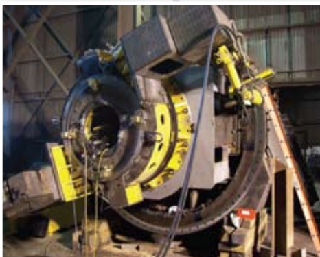
EAF Bearing Surface Machining
