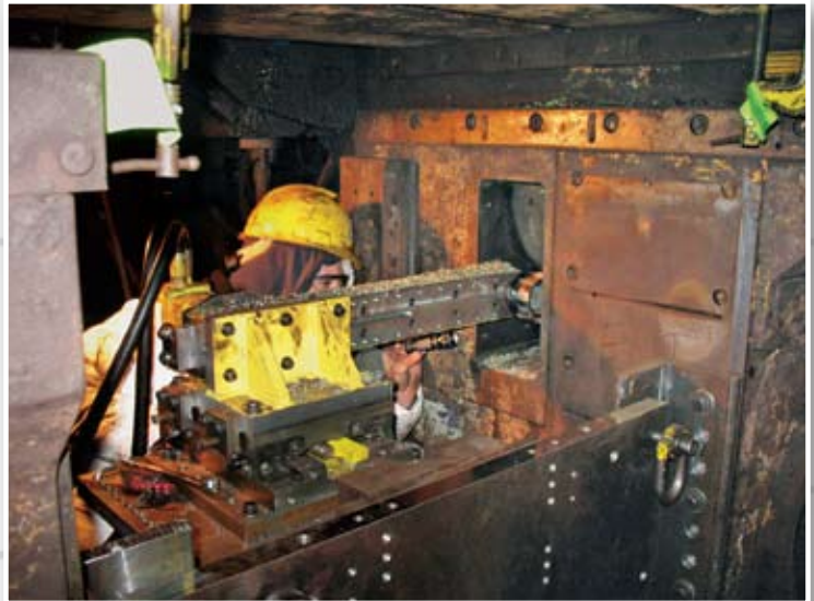
Machine Structural Mill Chock Keeper Slots
