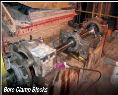
Machine Sag Mill End Flanges
