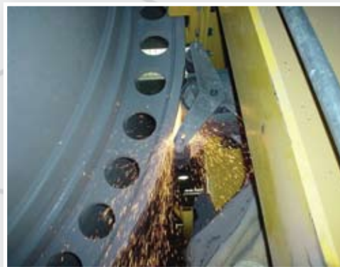
Grind Kiln Tires While in Operation
