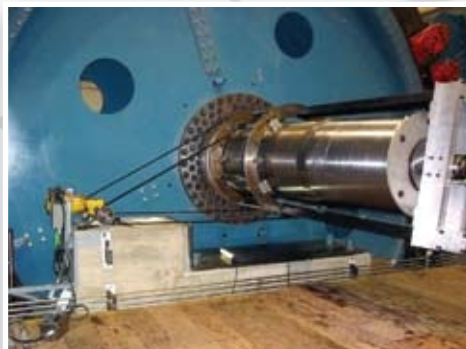
Refurbish Mine Hoist Tapered Journal
