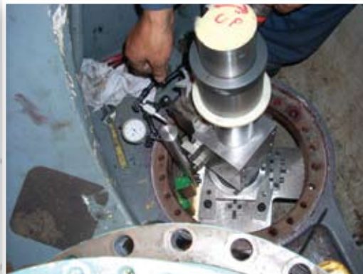
Repair and Reinforce Damaged Yaw Drive Flange
