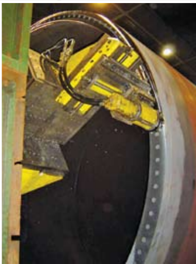
Tower Flange Machining
