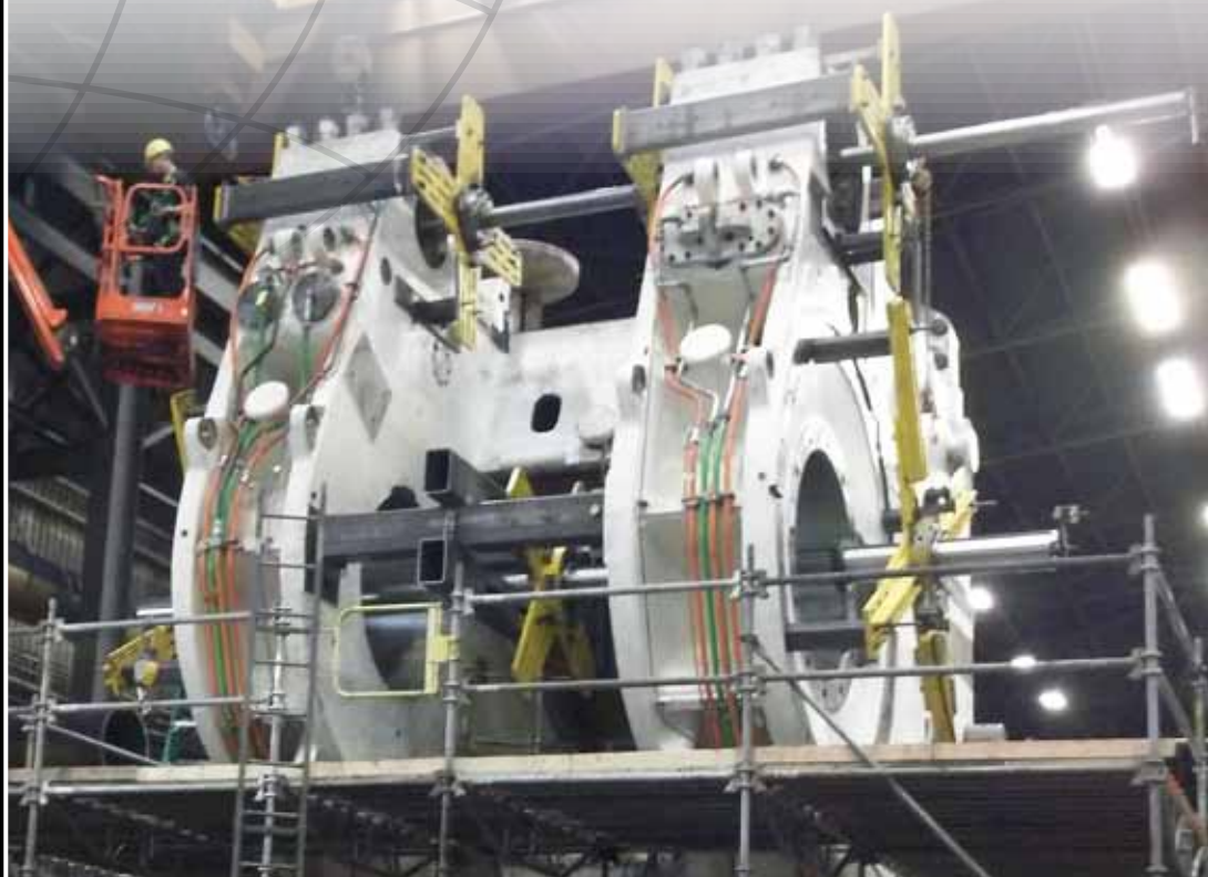
Machine Ram Seat Counterbore on Forging Press
