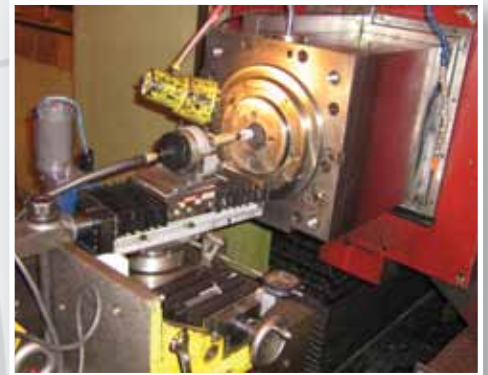
CNC Machining Center Spindle Grind
