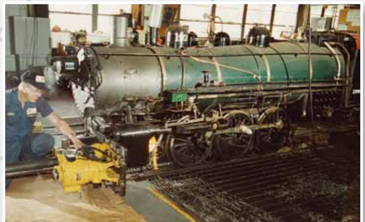
Steam Engine Cylinder Bore Repair
