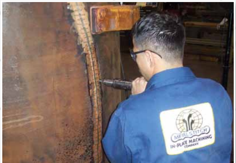
Metalstitch® Cold Cast Iron Repair
