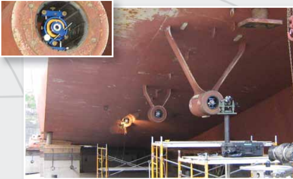
Inspect Alignment Between Propeller Strut Bores on Marine Vessel
