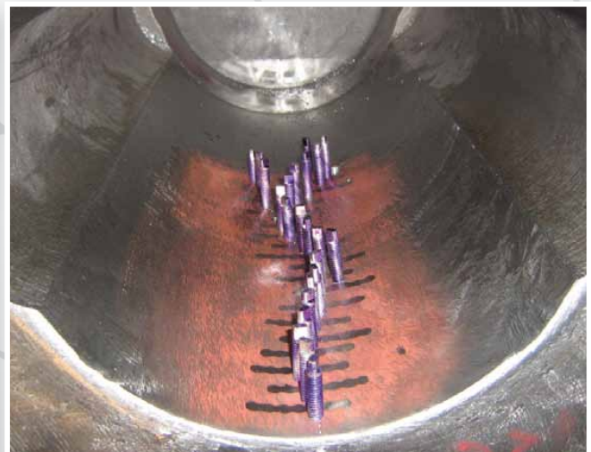
Extrusion Press Bore Metalstitch® Repair
