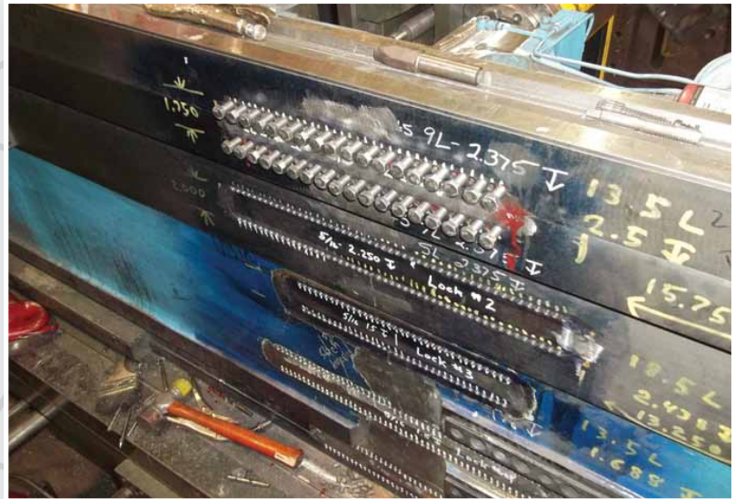
Installing Stitchscrew®, Stitchlock®, and Masterstitch® Components
