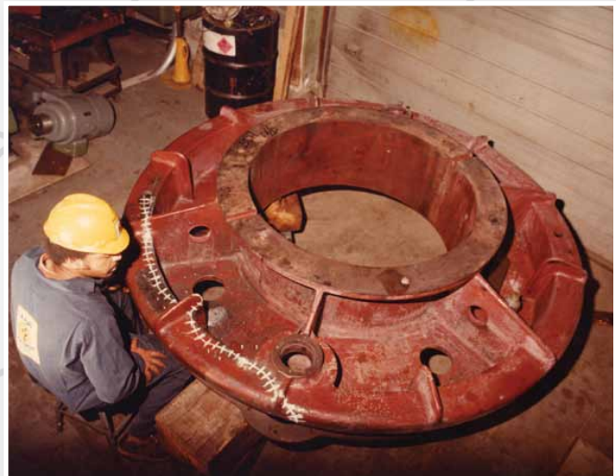
Hydro Cover Restored Using Metalstitch® Process
