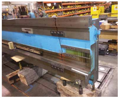
Cracked 25 Foot Gantry Mill Rail
