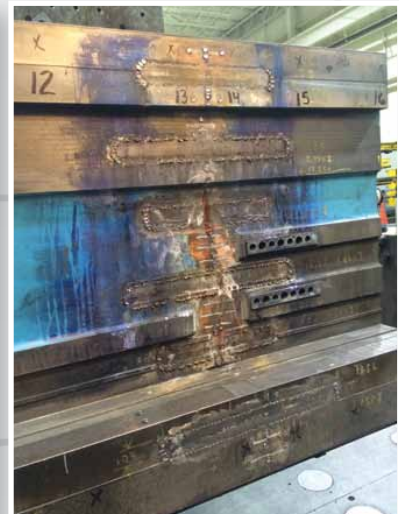
Metalstitch® Repair Ready for Machining
