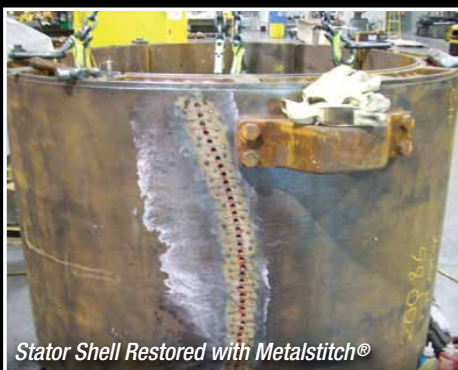
Metalstitch® Repair of Steam Turbine Shell
