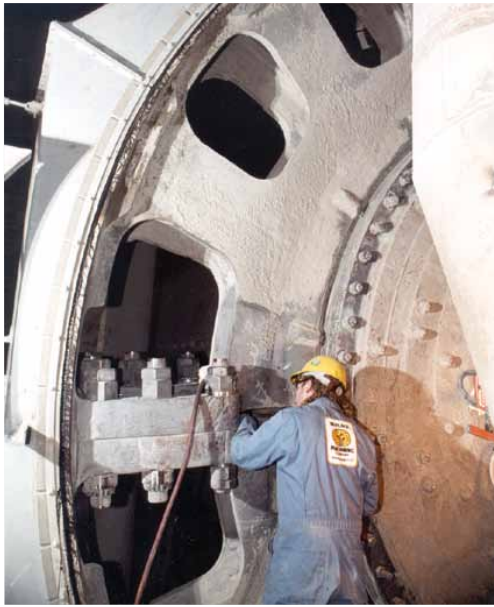
Ball Mill Metalstitch® Repair
