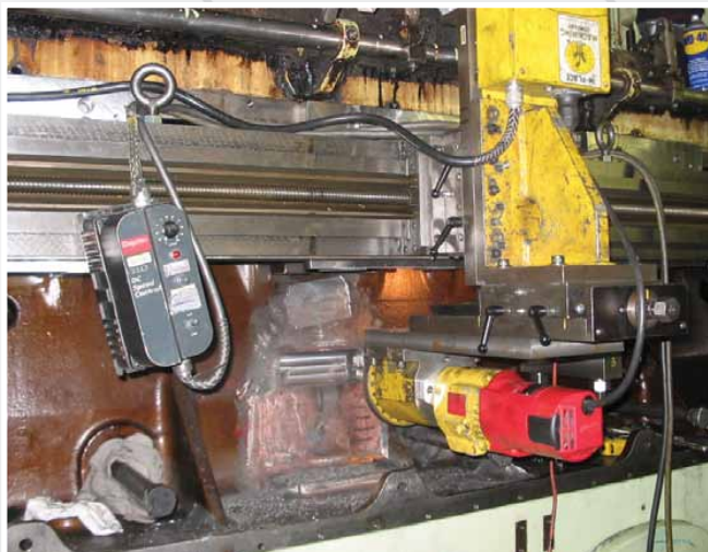
Machining Diesel Engine Insert After Metalstitch® Repair
