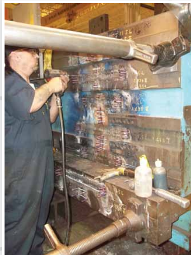
Inserting Stitchscrew® Components
