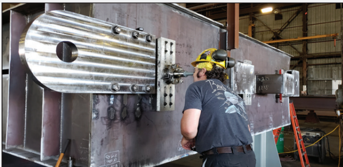
Optical Alignment of Line-Bore Bearings for Guide Wheel Bores
