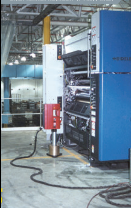
LASER TRACKER ALIGNMENT OF PRESS ROLLS
