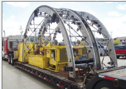
rotating the mill body. Once again IPM responded to industry demands for shorter outages and reduced maintenance spending with a unique on-site machining solution. The supersized system is In-Place Machining Company's latest addition to over 100 single point tooling, milling, grinding and honing systems based on planetary technology developed and perfected by the Company.
