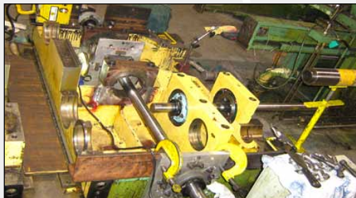
Setup for On-Site Line Boring
