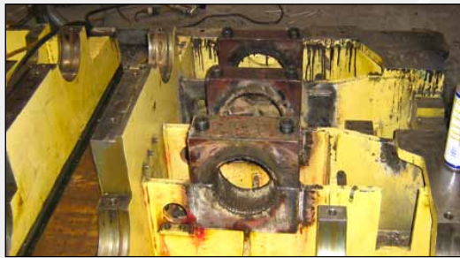
Gearbox Casing On-Site Machining
