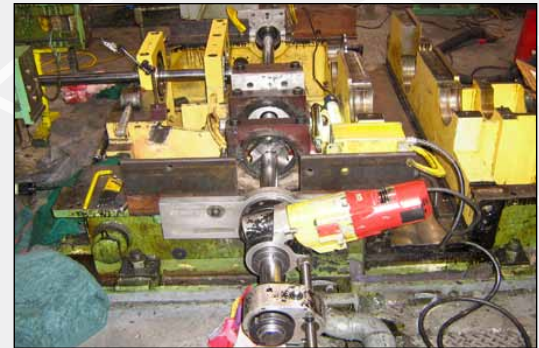
On-Site Line Boring Machining In Progress
