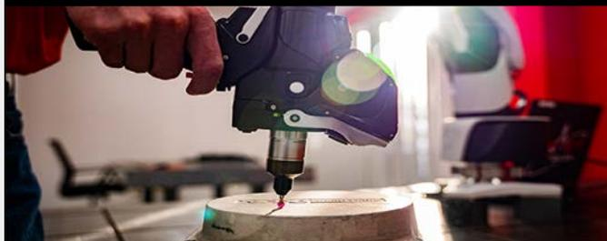
*Coordinate Measuring Machine (CMM) Probe*
