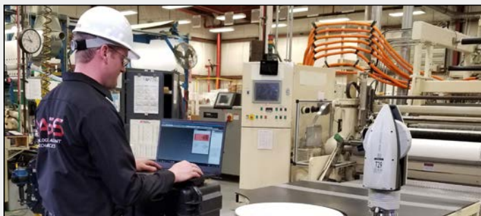
Laser Tracker Captures Roll Alignment Data
