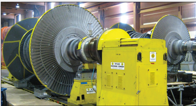
Portable Lathe - Blade Root Modification on 2 LP Rotors
